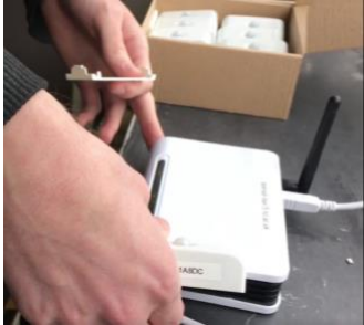
Figure 2: An auditor pairs an environment sensor with a base unit during deployment
